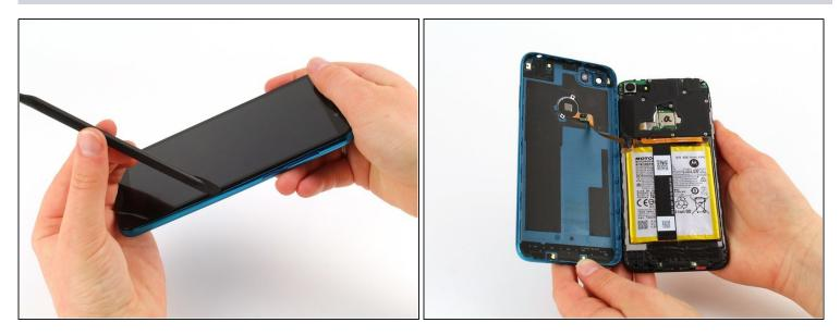
• Run the halberd spudger along the edges of the device. The back cover should easily pop off.
