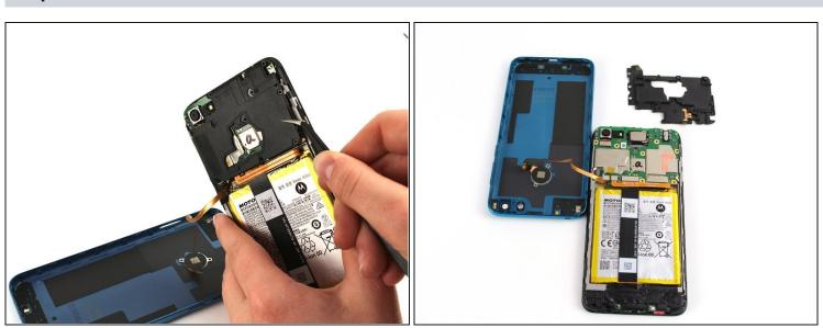
• With the angled tweezers, remove the black cover to reveal the motherboard underneath.
