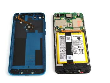
Use the angled tweezers to pry off the metal head of the connecting piece from the main motherboard assembly.
