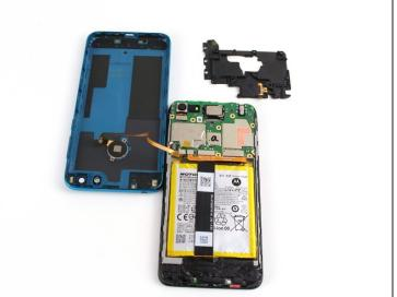
• With the angled tweezers, remove the black cover to reveal the motherboard underneath.
