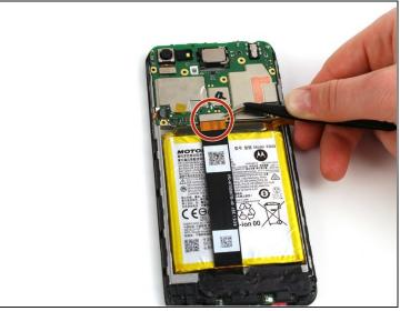
Using the angled tweezers, detach the two connectors from the motherboard by pulling the metallic heads up and away from the phone.
