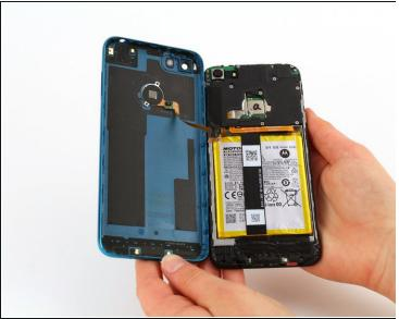
Run the halberd spudger along the edges of the device. The back cover should easily pop off.
