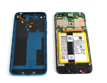
Use the angled tweezers to pry off the metal head of the connecting piece from the main motherboard assembly.
