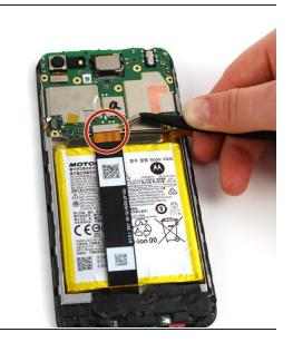
Using the angled tweezers, detach the two connectors from the motherboard by pulling the metallic head up and away from the phone.
