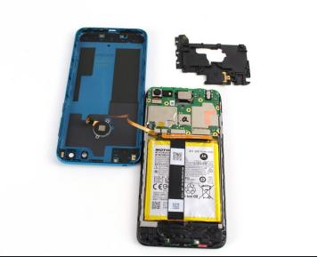
With the angled tweezers, remove the black cover to reveal the motherboard underneath.
