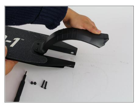
• Pull the foot brake/ wheel cover away from the deck and downwards.
