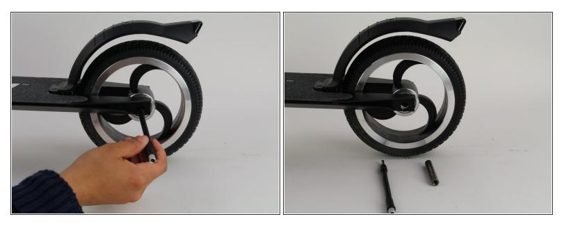
• Use a 4 mm bit extension to push the axle out of the wheel's center.
