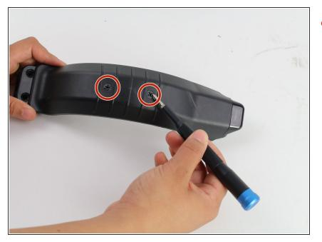
On the foot brake, remove the two
