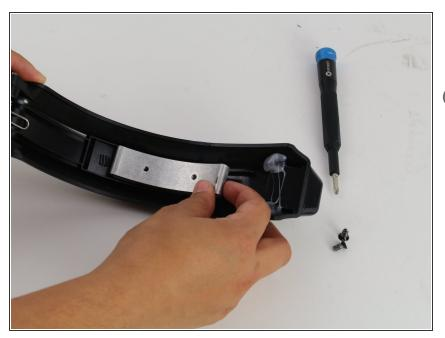
• On the opposite side of the brake, remove the silver brake pad.
