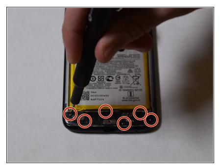
Remove the six 3.2 mm screws from the charging port assembly cover with a Phillips #00 screwdriver.
