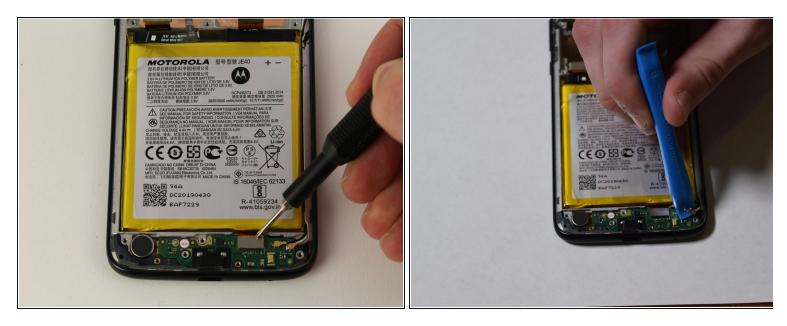
• Using an iFixit opening tool, detach the cables from the charging port assembly.
