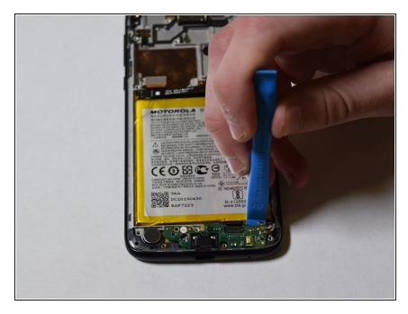
Using the iFixit opening tool, carefully pry up the charging port assembly.
