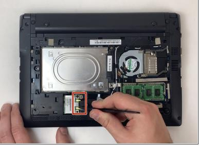
Use tweezers to disconnect the black and white wires from the wireless card by pulling them up off the card.
