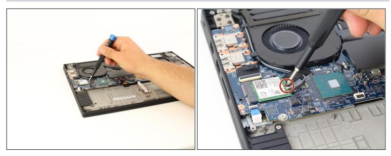
• Using a Phillips #00 head screwdriver, remove the 3mm screw holding the wireless adapter to the motherboard.
