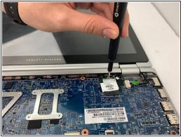
Take the #1 Phillips screwdriver and unscrew the 0.4mm silver screw holding down the wireless card.
