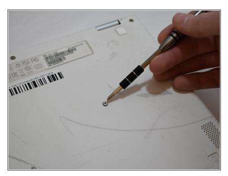
Remove eleven 7.2 mm screws from the bottom of the Chromebook using a JIS #1 screwdriver.
