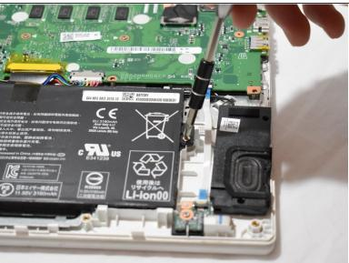
Remove two 4.6 mm JIS # screws at each end of the battery.
