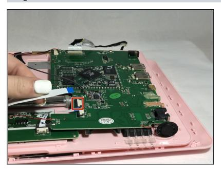
Disconnect the black connectors from the motherboard by pulling on the white ribbon cable.
