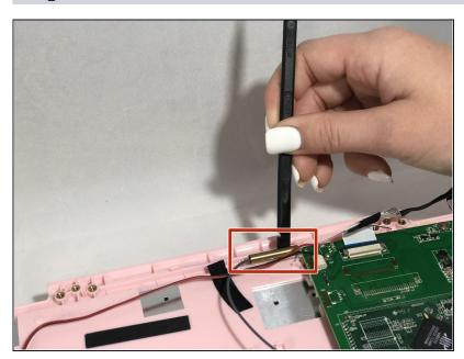
Using a spudger, remove the gold cylinder out of the indent at the bottom of the computer.
