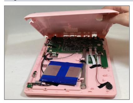
Remove the bottom of the netbook by lifting the corners.
