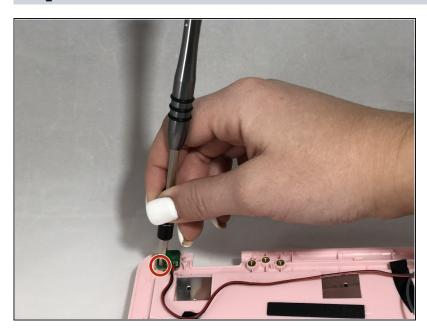
Remove the two 6mm silver screws from the small circuit board connected to the motherboard by the red and black wires.
