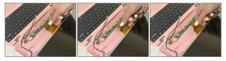
• Detach the wide yellow ribbon cable connected to the screen from the computer.
