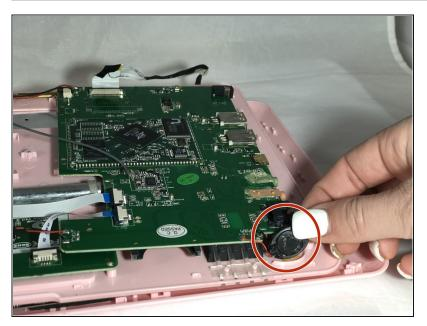
Remove the two small black speakers on the corners connected to the motherboard by the black and red wires.
