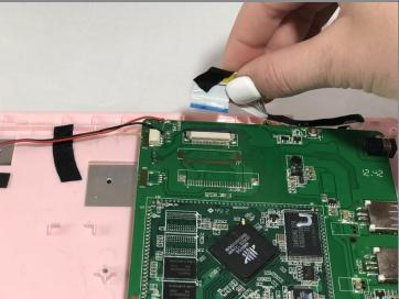
• Remove the black covered wire connected to the motherboard by pulling the white ribbon cable away from the motherboard.
