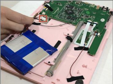
• Pinch the red and black wires connected to the section closest to the small white connector, and pull to remove them from the motherboard.
