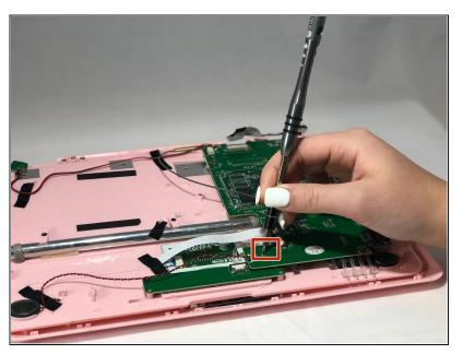
Remove the six 6mm Phillips #00 screws from the motherboard.
