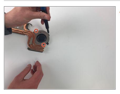
Remove the three 3.5 mm screws on each fan holding the fan to the heat sink using a Phillips #0 screwdriver.
