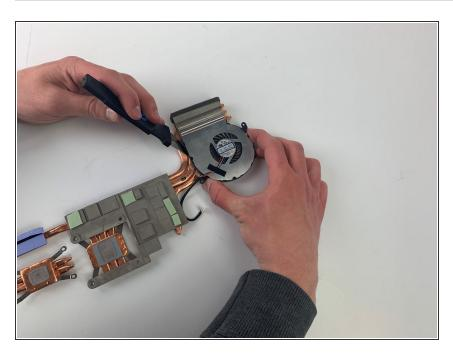
Separate the heat sink from the tab on the side holding the fan in place.
