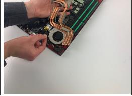
Using the Jimmy tool, remove the adhesive pads securing the fans to the board.
