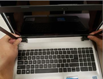
Unsnap the two hinges attached to the clam shell by pulling towards yourself and then up.
