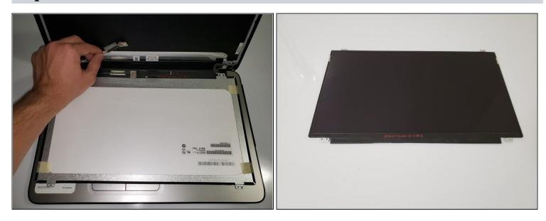
• Gently disconnect the video cable to detach the LCD screen from the back panel.
