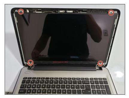
Remove the four 3mm screws that are holding the LCD panel in place.
