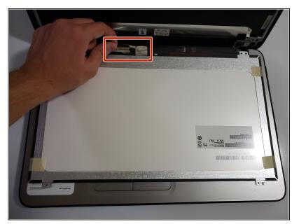
• Peel the tape securing the video cable.
