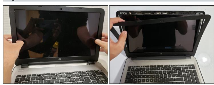
• Gently pull away the bezel by the inner edge starting from the side until bezel is detached from screen.
