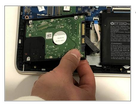
Lift the hard drive out of its enclosure and take off the plastic/rubber siding used to secure the hard drive in place.
