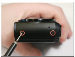
Remove the six 4mm screws located on the side and bottom of the camera casing using a Phillips #000 screwdriver.
