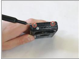
Remove the four 2mm Phillips #000 screws on the sides of the exposed internal metal plate within the camera.
