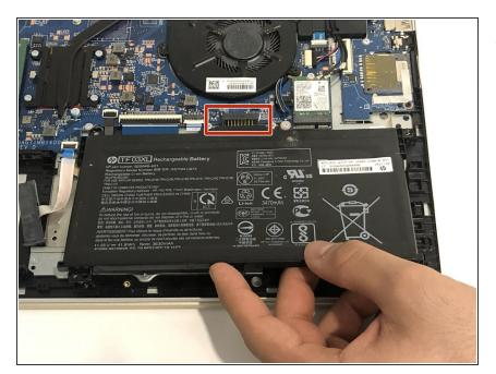
Lift the battery up and away from the battery pins.
