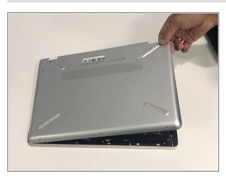
Carefully remove the back plate from the laptop.
