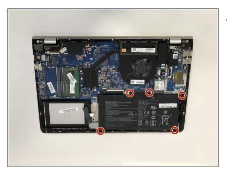
Remove the five 5mm Phillips #1 screws surrounding the battery.
