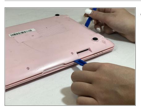
Using two plastic opening tools, pry off the bottom of the netbook by going around the edges.
