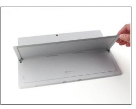
Lift the kickstand to expose the hinge screws.
