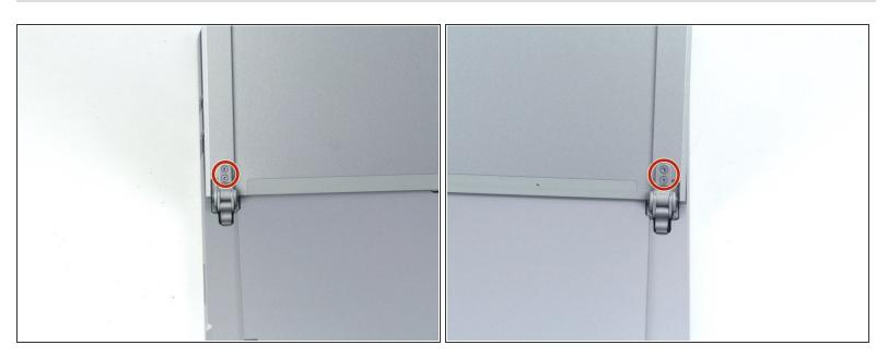
• Remove the four 2.7 mm T3 screws—two on each side of the kickstand.
