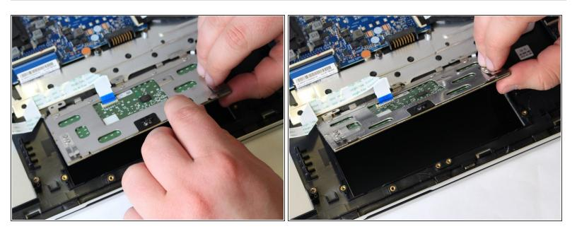
Remove the trackpad from the device, lifting the bottom edge first.
