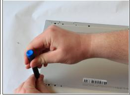
Using the Phillips #0 screwdriver, remove the seven 5mm screws from the back case.
