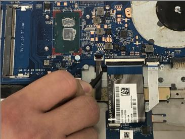
• Remove the nine cables from the motherboard by carefully lifting the black tab on each connector.
