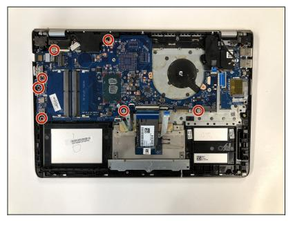
Remove the seven screws from the motherboard using a JIS #1 screwdriver.
