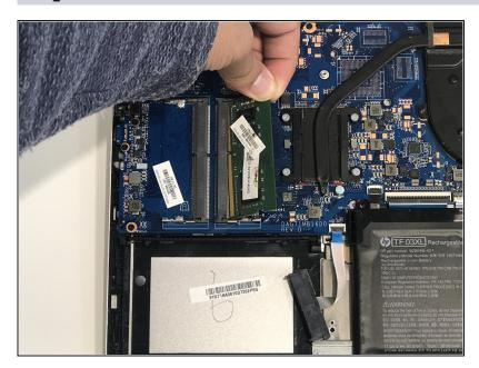
• Remove the card by pulling it up and away from the slot.
