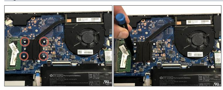
• Remove the four 2.9mm JIS #1 screws from each of the four corners of the fan.
