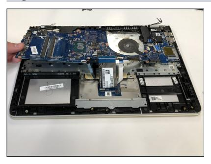
Carefully remove the motherboard from the casing.
