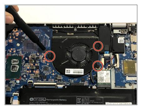
Remove the three 2.9mm JIS #1 screws surrounding the fan.
