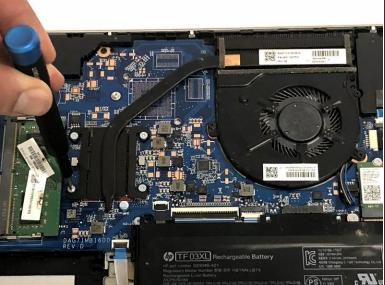
• Remove the four 2.9mm JIS #1 screws from each of the four corners of the fan.
