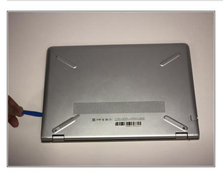
Unclip the back plate using a plastic opening tool.
