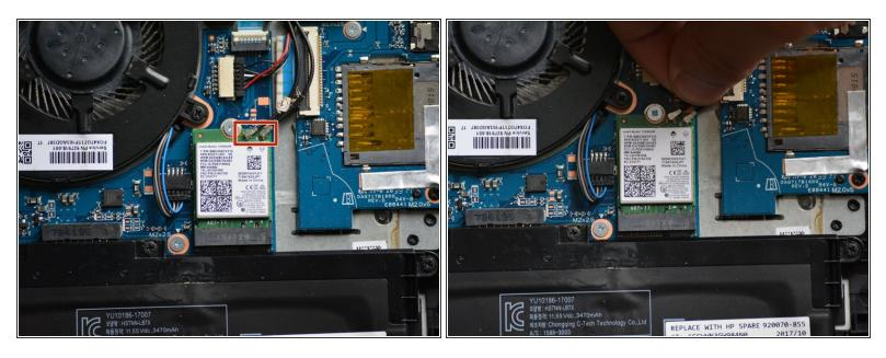
• Disconnect the two Wi-Fi and Bluetooth antenna wires by gently pulling them away from the board.
