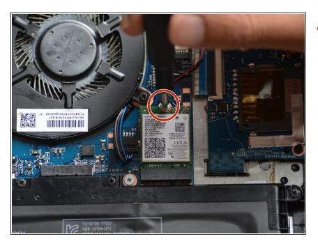
Remove the JIS #1 screw from the WLAN card.
