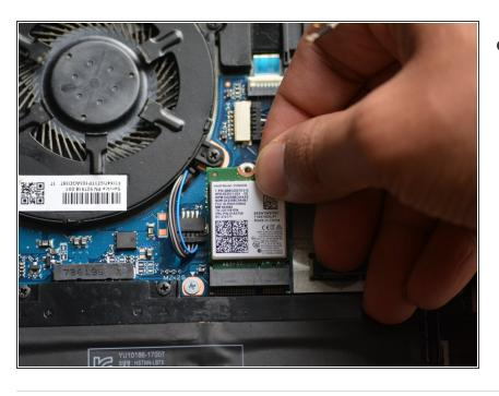
Remove the card by pulling it away from the slot.
