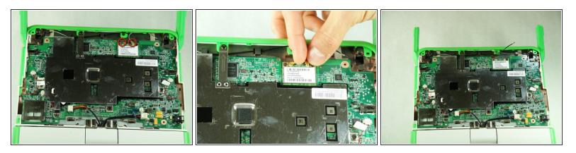
Mhen pulling out the connectors, make sure to hold the metal connector instead of the wire.
