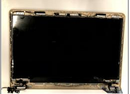
Use the metal spudger to carefully pry off the plastic encasing around the monitor.
