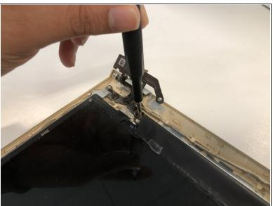
Remove the four JIS #1 screws holding the screen in place.
