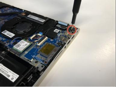
Remove the five JIS #1 screws that attach the hinges of the screen to the casing of the laptop.
