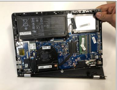
Carefully lift the hinges from the encasing and lift the bottom half of the laptop away from the screen.
