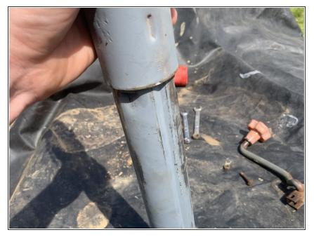
• During re-assembly, align the notch on the upper assembly to the grove on the lower assembly.
