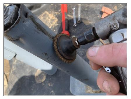
Remove rust and corrosion from the upper and lower assemblies of the jack using a die-grinder and sanding pad.
