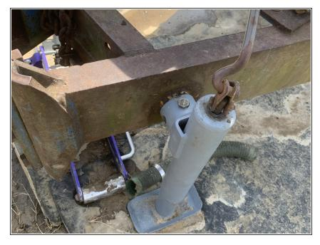
• Install the jack to the trailer and test for correct operation.
