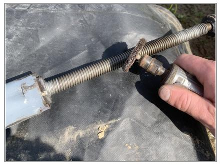
Begin to remove the rust and corrosion using a die-grinder and steel wire wheel.
