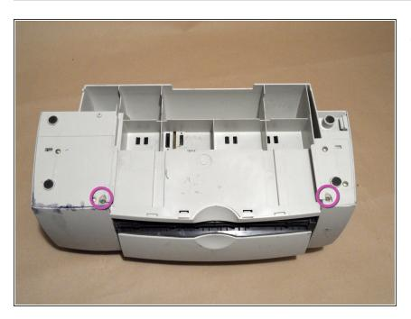
Additionally, remove those two screws at the bottom of the device.
