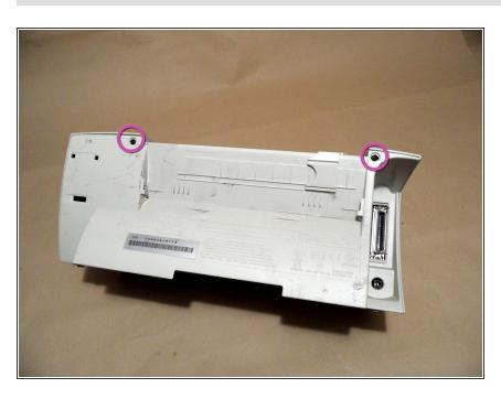
To remove the cover and housing use a screw driver to remove the highlighted screws.
