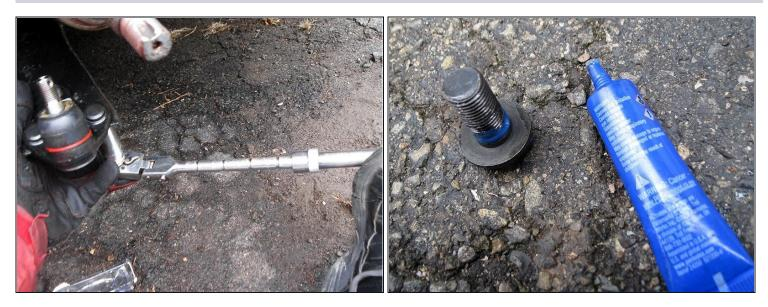
• Mount the new ball joint, I put a little Blue Thread Lock on the bolt, the nuts had nylon inserts.
