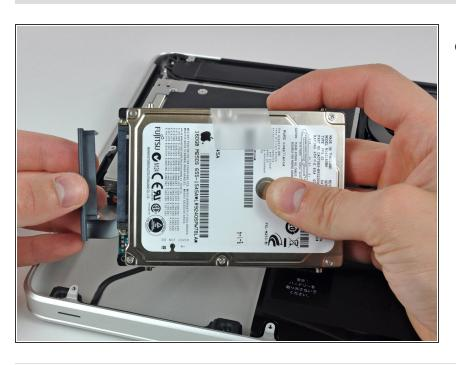
Remove the hard drive cable by pulling its connector straight away from the hard drive.
