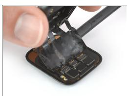
• Lift the body of the watch up and carefully slide a spudger underneath the display flex cable to loosen remaining adhesive.
