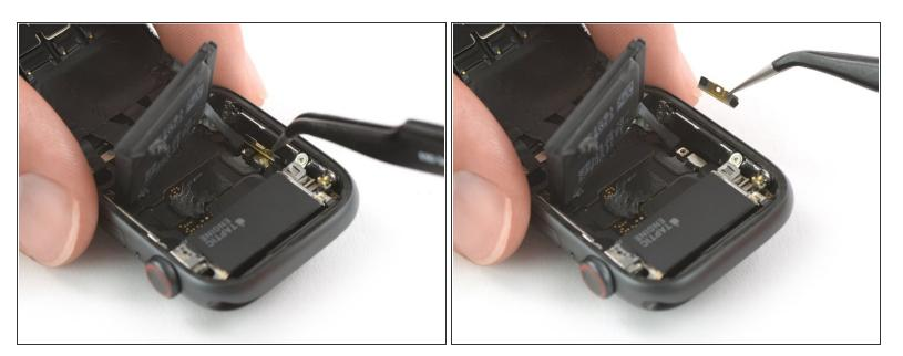
Use a pair of tweezers to remove the metal plate which covers the battery connector.
