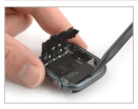
Use the pointed end of a spudger to make final position adjustments and press the adhesive into place.
