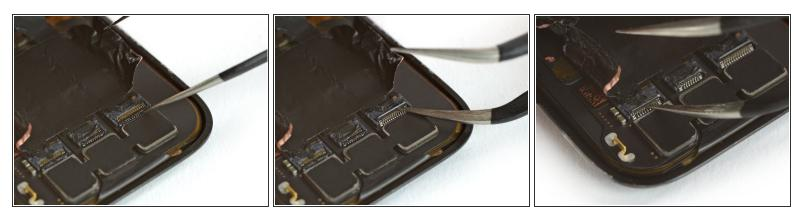
Use one arm of a pair of tweezers to carfully open the three ZIF connectors on the rear side of the screen.
