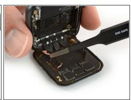
• Use a pair of blunt nose tweezers to peel up the sides of the black foil which adheres the cable to the rear side of the screen.
