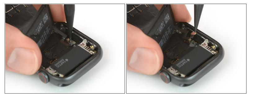
Use the pointed end of a spudger to pry up and disconnect the battery flex cable.
