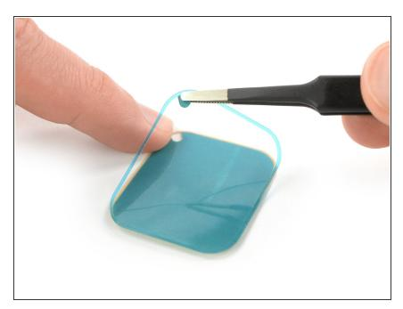
Use a pair of tweezers to carefully remove the replacement adhesive with the blue protective film from the backing paper.
