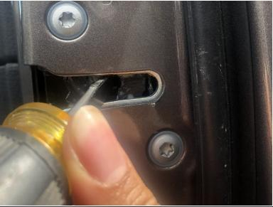
• While the exterior door handle is being pulled, push the screwdriver against the left leg of the latch.
