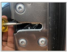
Use the screwdriver to push the latch upwards into the final unlocked position.
