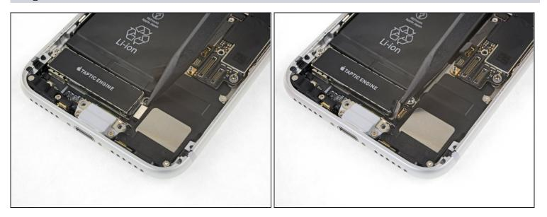
• Use the point of your spudger to pry up and disconnect the Taptic Engine flex cable.
