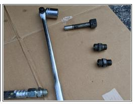
After the first fitting was off, I was able to get a 24 mm socket over the second one to remove the fitting.
