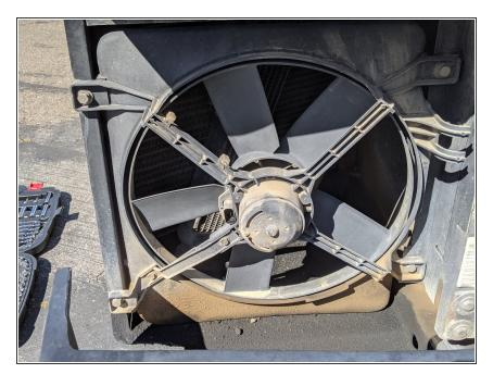
There's one electrical plug and 4 obvious hex bolts to remove the condenser fan.
