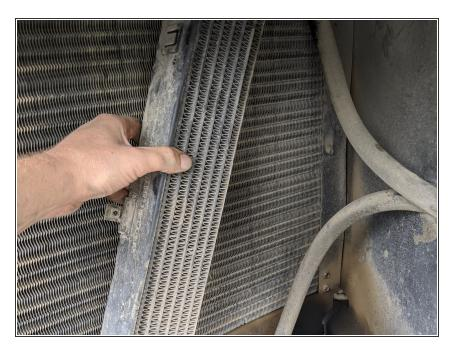
Getting the oil cooler off the condenser was easy, there's just two bolts. But it's still attached to the engine...
