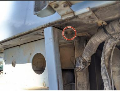
On my Vixen there was a hex head bolt on the top right, and a on-its-way-to-being-stripped Phillips head bolt on the top left.
