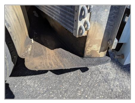
After removing the side panel, it's clear that my oil cooler has been leaking for a while. Fortunately, AFAB sells a <u>complete replacement</u> <u>kit</u> including a new oil cooler and new hoses!
