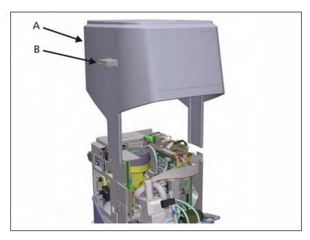
Lift the Main Cover (A) from the Ventilation Unit using the Standoff Brackets (B) attached to the Main Cover.
