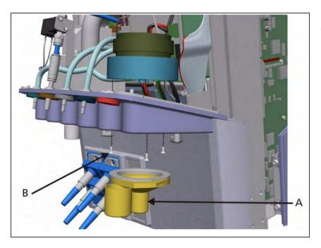
Disconnect 2 cables from the magnet of the Expiratory Valve.
