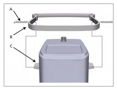
Remove 4 Hex Allen screws (A) from the Rail surrounding the Ventilation Unit.
