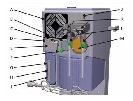
Remove the fan filter (A). No tools should be necessary.
