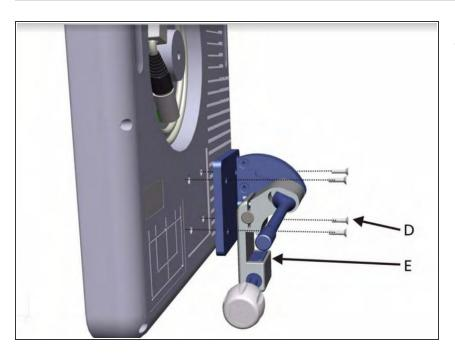
• Remove the 4 screws (D) to remove the panel's swivel mount (E).
