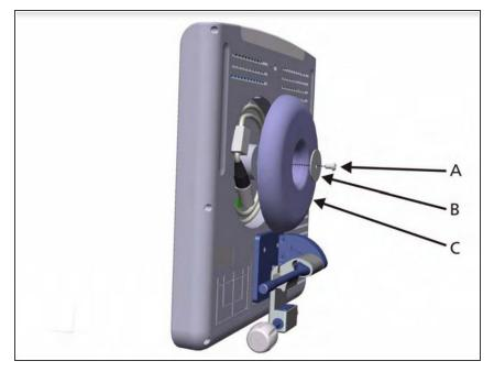
Remove the screw (A) and washer(B) and remove the cable management cover (C).
