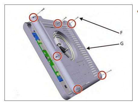
Remove the 6 screws (F) and remove the back panel (G).
