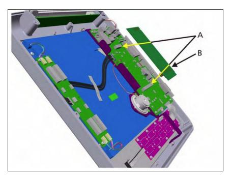
If nessesary, remove the ESM module by disconnecting the module from the connecting sockets (A).
