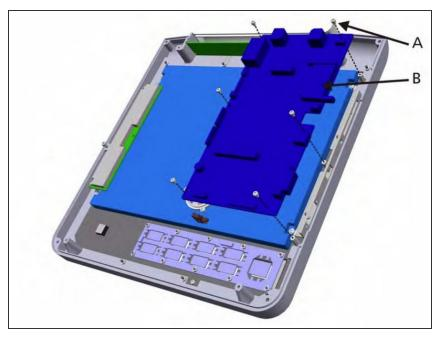
• Remove the 3 screws and 3 nuts, then lift out the motherboard.
