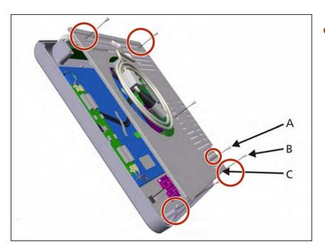
• Remove the 5 screws and remove the metal shield.
