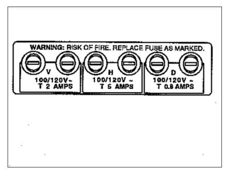
Use a screwdriver to push in and turn the fuse holder counterclockwise until it disengages.
