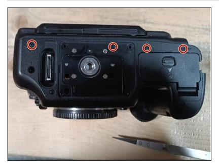
Remove the 4 screws (1 was under the plate removed under the last step)
