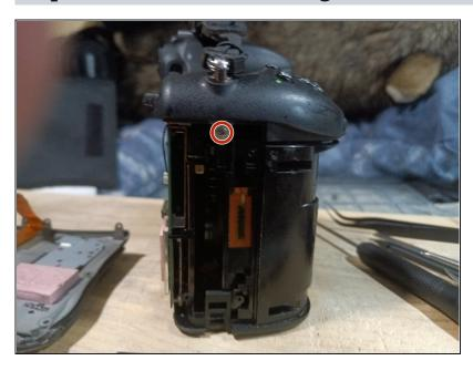
Remove the screw that had been hidden under the memory slot cover.
