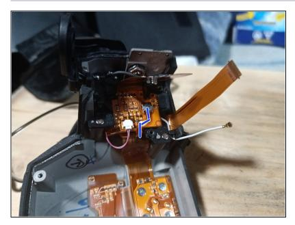
Once unfolded, Locate the white socket with the tiny ribbon cable (it's about about 4 mm wide), cable highlighted with blue
