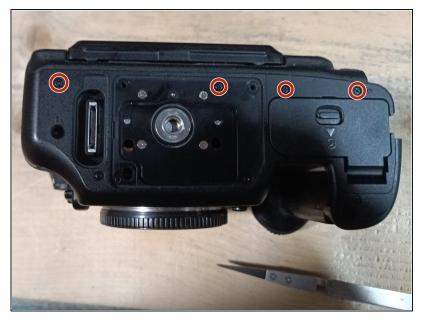
• Remove the 4 screws (1 was under the plate removed under the last step)
