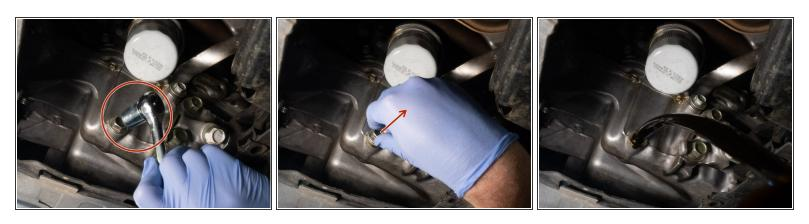
Remove the drain bolt with a 17mm socket wrench, and completely drain the oil.
