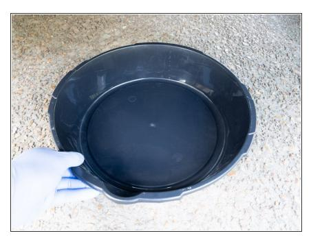
Place the drain pain under the chassis and align with the drain bolt.
