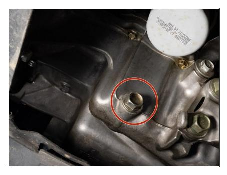
Locate the drain bolt.
