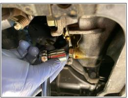
Replace the drain bolt with a new drain bolt gasket (crush washer); Honda Washer, Drain Plug (14MM) 94109-14000. Use the 17mm socket wrench to tighten.
