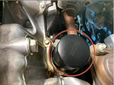
Install the new filter in place of the old filter. Hand tighten instead of using the oil filter wrench.
