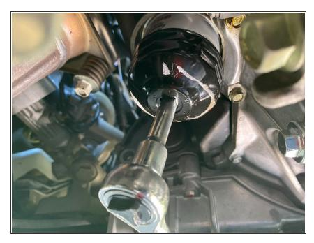
Remove the oil filter with a 45mm oil filter socket.
