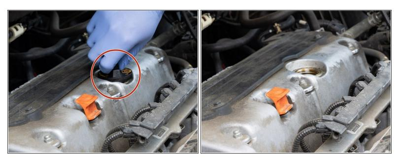
Let the vehicle cool for 15 minutes if needed. Clean the area around the oil cap. Remove the oil cap.
