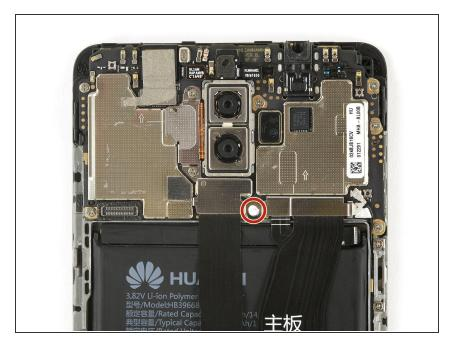
Remove the water indicator sticker and the Phillips #00 screw beneath it, that holds the cable bracket in its place.
