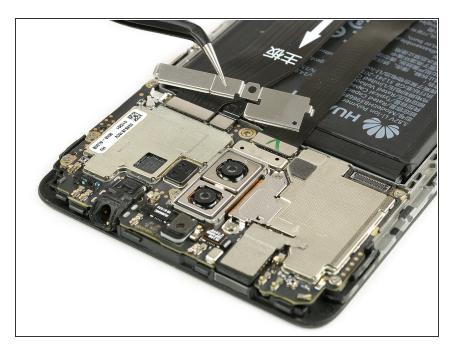
Remove the cable bracket.
