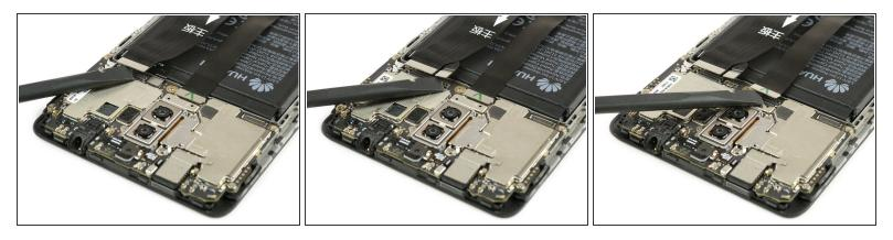
• Use a spudger to disconnect the interconnect, the battery and the display flex cable.
