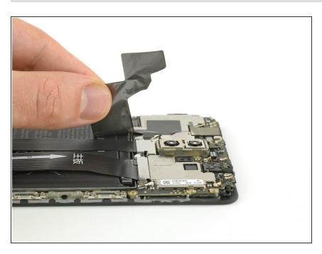
Carefully peel off the plastic sticker that holds both cables to the battery.
