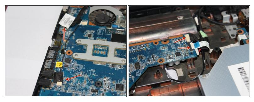
• Remove the 3 Display Cables and a USB Port Ribbon Cable
