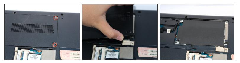
• Remove 2 Screw from the Hard Drive Cover and lift up the cover
