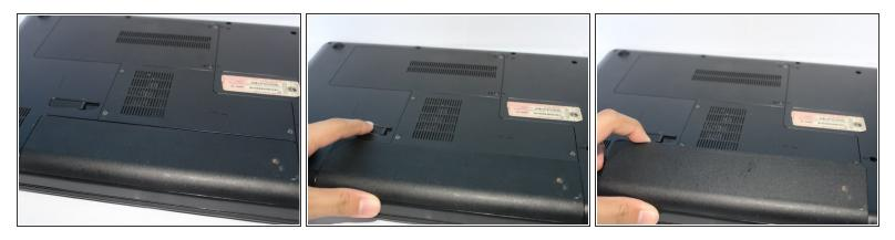
• Remove Battery by sliding the tab
