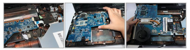
• Remove the Power Cable and pull the motherboard to the right
