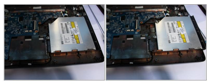
Remove the CD Drive by Pushing or Pulling to the outside
