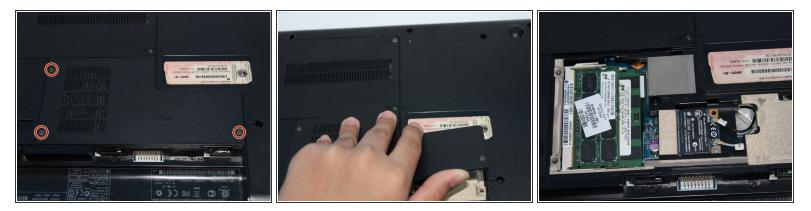
Remove the 3 screws from the Ram Cover and lift up the cover
