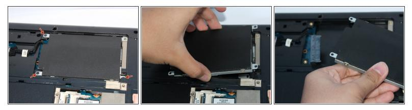
• Remove the 3 screws from the Hard Drive
