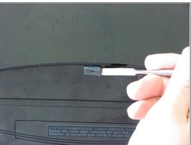
Remove the rubber screw cover near the hard drive cover with a spudger.
