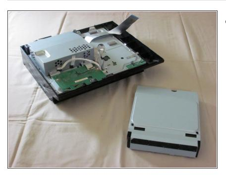
Remove the optical drive enclosure from the PS3.
