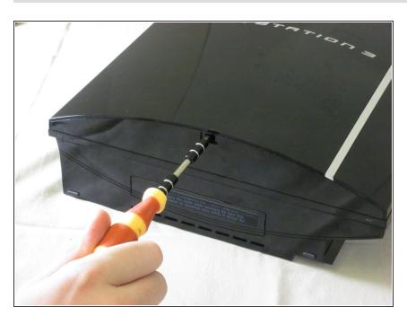
Remove the screw holding the top cover in place with a Torx T10 screwdriver.
