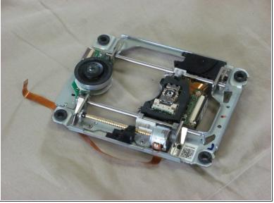
Carefully lift the optical drive out of the enclosure.
