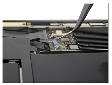
• Peel back the tape covering the battery connector enough to reveal the connector underneath.
