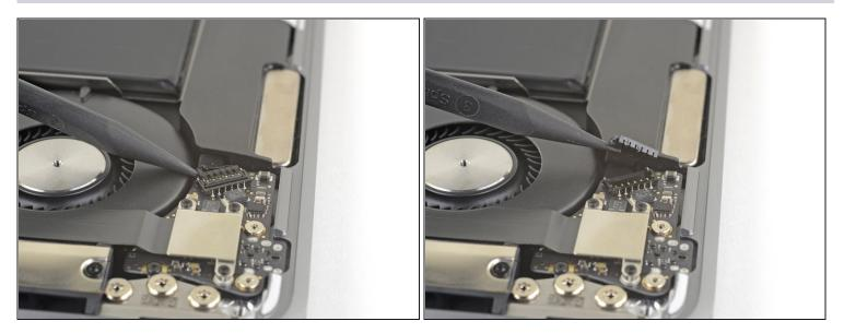
• Slide the tip of a spudger underneath the right speaker cable and pry straight up to disconnect the speaker.
