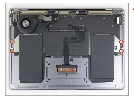
• Use a T3 Torx driver to remove four 2.5 mm screws securing the battery.
