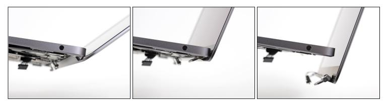
• Lift the MacBook and carefully rotate the display to a 90 degree angle with the upper case.
