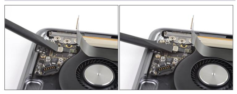
• Use the flat end of a spudger to pry the Touch ID sensor connector straight up and disconnect it.
