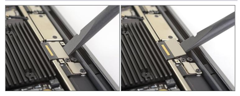
• Use the flat end of a spudger to pry up the display cable connector.
