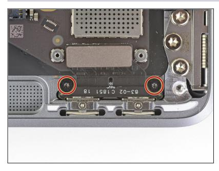
• Use a T4 Torx driver to remove the two 2.9 mm screws securing the USB-C board.
