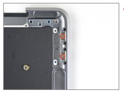
• Use a P2 pentalobe driver to remove the two 1.1 mm screws securing the USB-C port brackets.
