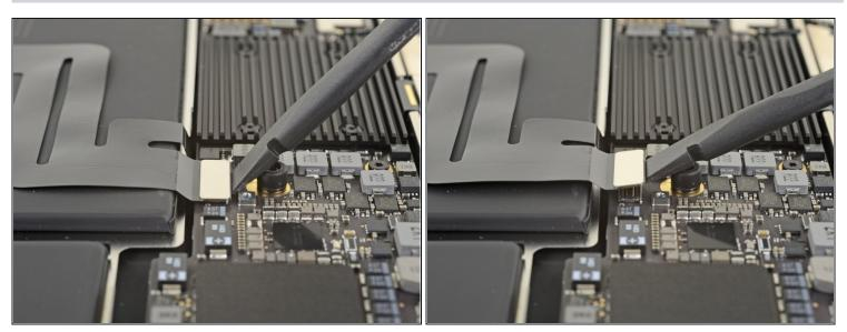
• Use the flat end of a spudger to pry the trackpad cable connector up and out of its socket.
