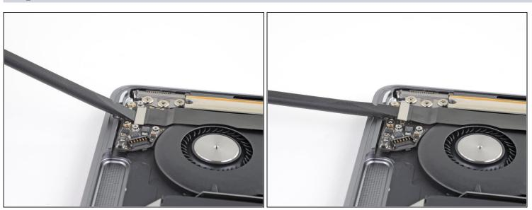
• Use the flat end of a spudger to pry the audio board connector straight up and disconnect it.
