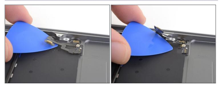
• Slide an opening pick under the rest of the microphone assembly cable to separate it from the adhesive securing it to the upper case.
