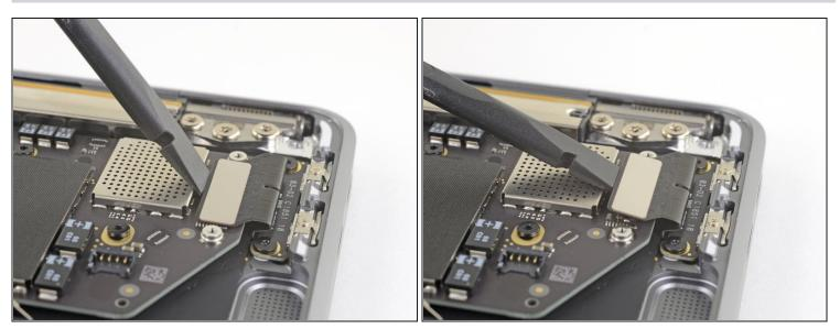
• Use the flat end of a spudger to pry the USB-C cable connector up and out of its socket on the logic board.
