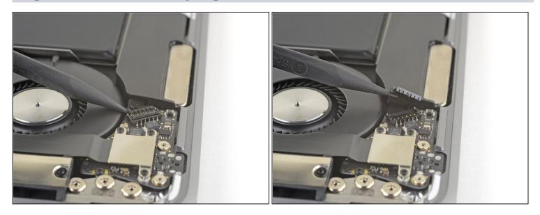
• Slide the tip of a spudger underneath the speaker cable and pry straight up to disconnect the speaker.
