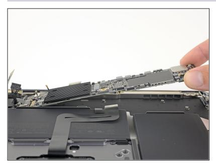
• Remove the logic board.
