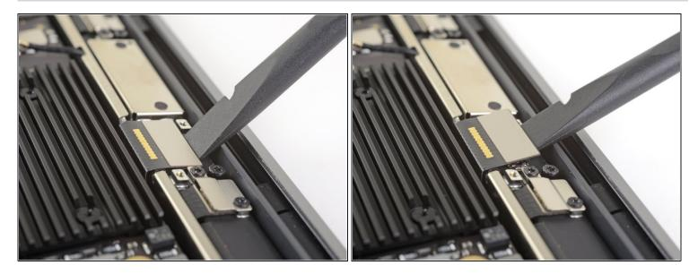
• Use the flat end of a spudger to pry up the display cable connector.
