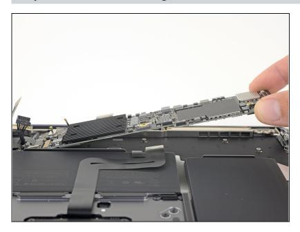
• Remove the logic board.
