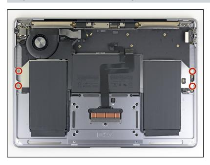
Use a T3 Torx driver to remove four 2.5 mm screws securing the battery.
