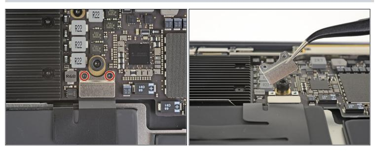
Use a T3 Torx driver to remove the two 1.4 mm screws securing the trackpad connector bracket.
