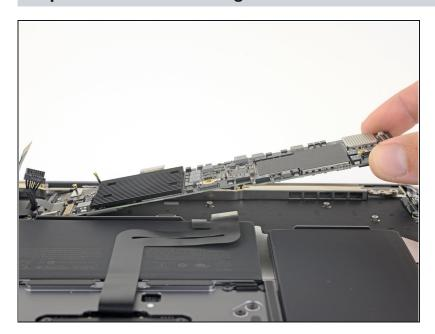
• Remove the logic board.
