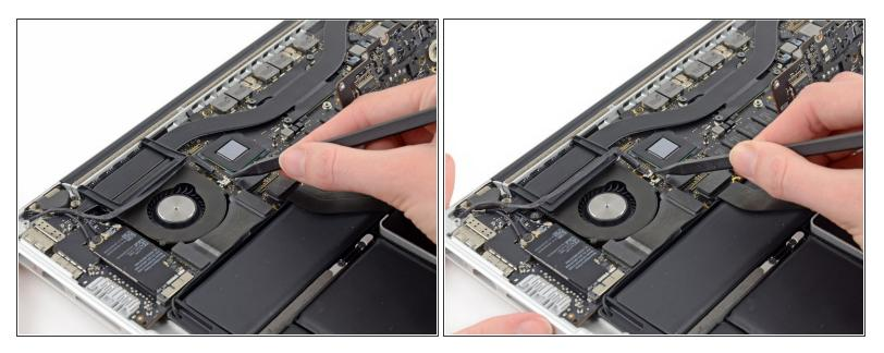
Use the tip of a spudger to push the iSight camera cable connector straight away from its socket on the logic board.
