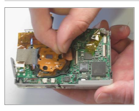
Remove lens data cable by gently pulling it out.
