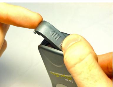
Flip the device so that the bottom is facing upwards. Using thumb, push the tab on the bottom in the direction indicated by the arrow and then lift the unhinged part of the tab.
