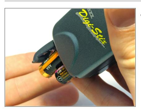
Tilt device so that batteries slide out.
